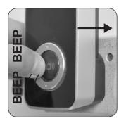
On each receiver, SELECT and HOLD the 'Chime Selection' Button for 10 SECONDS. An audible beep will be heard. The receiver is now in a waiting mode.
