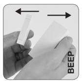
**PRESS** the bell push or ACTIVATE the magnetic sensor by separating the magnet from the sensor. An audible beep will be heard again from the receiver. The receiver is now being programmed.
