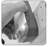
4 CONTINUE to HOLD the Chime Selection Button for 10 SECONDS, after which the strobe will flash or an audible beep will sound, indicating that the memory is now clear and ready for programming.
