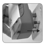
3 STILL HOLDING the Chime Selection Button, SWITCH the power back on by INSERTING the plug into the mains supply.
