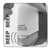
**1** PRESS and HOLD the chime selection button on the signal booster for 10 seconds until an audible beep beep is heard. The signal booster is now in waiting mode.
