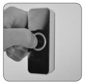
**2** PRESS the bell push. An audible single beep will be heard again from the receiver. The receiver is now being programmed.
