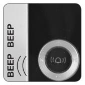
To exit the programming mode, PRESS the chime selection button again or WAIT a further 10 SECONDS until a beep beep is heard and the programming is finished. You are now linked!
