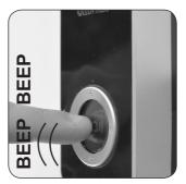
On each receiver, PRESS and HOLD the chime selection button for 10 SECONDS. An audible beep beep will be heard. The receiver is now in a waiting mode.
