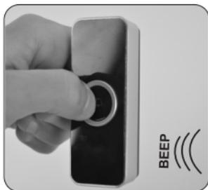
**1.** On each chime unit, press and hold the chime replay ► button for 10 seconds. An audible beep beep will be heard. The chime unit is now in a waiting mode for 15 seconds to link the transmitter.
