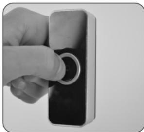
**3.** To exit programming mode, press the chime replay ► button again or wait several seconds until a beep beep is heard. The link process has now completed.
