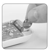
**2 REMOVE** the plastic tab located at the battery connector and **DISCARD** of it safely. The distress button will not work if the tab is not removed.
