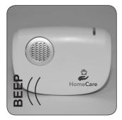
**3** To exit the programming mode, **PRESS** the chime replay button again or **WAIT** a further **10 SECONDS** until a beep is heard and the programming is finished.
