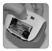
3 STILL HOLDING the chime replay button, SWITCH the power back on by INSERTING the batteries.
