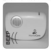
On each receiver, PRESS and HOLD the chime replay button for 10 SECONDS. An audible beep will be heard. The receiver is now in a waiting mode.
