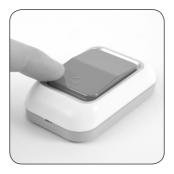
**2** PRESS the distress button. An audible beep will be heard again from the receiver. The receiver is now being programmed.
