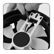
10 ENSURE that the wires are TUCKED into the slot provided (as shown). Failure to do this will result in the blades hitting the wires during operation.
