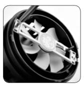
11 USE a cross headed screwdriver to REATTACH the screws holding in the frame for the fan blades.
