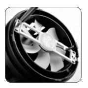
USE a cross headed screwdriver (Not Included) to **REMOVE** the screws at either side of the frame.
