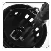
USE a cross headed screwdriver to REMOVE the screw holding the UV lamp in place.
