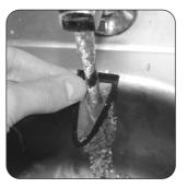
**2** RINSE the filter under warm water to remove any deposits. DRY THOROUGHLY before re-use.
