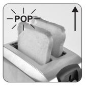
Toasting will continue for a period of time set by the browning control. Once toasting has completed, the carriage lever will automatically release and the toasted bread will 'POP' out of the toasting slots. The heating element will automatically switch 'off' at this stage.
