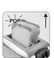
Once toasting has completed, the carriage lever will automatically release and the toasted bread will 'POP' out of the toasting slots. The heating element will automatically switch 'off' at this stage.
