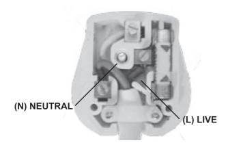
Your appliance operates on 220-240V~50Hz AC Mains and comes fitted with a 3-pin BSI Approved plug, so that it is ready for use for the UK or Eire market. If for any reason you need to fit a new plug, the flexible mains lead must be connected as shown below: -
