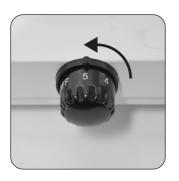
TURN the adjustable temperature control dial ANTI-CLOCKWISE from the 'off' position to the required temperature setting. If you need a HIGH HEAT, TURN the dial, to MAX. To operate at LOW or MEDIUM HEATS, TURN the dial to any of the other settings ACCORDINGLY.
