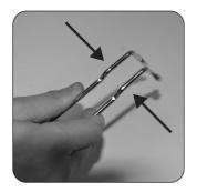
1 SQUEEZE the prongs on the handle TOGETHER and HOLD that position.
