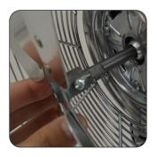
**4.** Remove the black rubber protector from the shaft. Carefully handle the fan blades and loosen the small screw at the back of the blades. No need to remove. Now slide the blades onto the shaft so that the screw is positioned over the flat notch in the shaft and tighten the screw so that the blades are tight onto the shaft.
