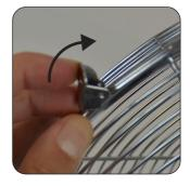
**6.** Open the four clamps on the front grille. Position the front part grille with the V shaped notch at the top and there will be two tiny holes at the bottom which will require alignment. Close the 4 clamps so that they clamp to the back grille and hold it tight together.
