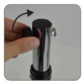
**3.** Now stand the base on the floor. At top of the long tube unscrew the other knob and bolt. One end of the bolt has a squared flange.
