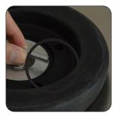
**13.** With the two small holes at the bottom of the grills aligned, insert the tiny nut and bolt through the holes and tighten.
