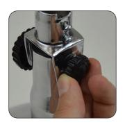
7. Replace the small grub screw which should now tighten against the oval groove. On the opposite side replace the small black screw which will tighten in the oval hole. This stops the head of the fan from tilting too far up or down.
