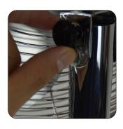
**9.** Put the knob back on the bolt and tighten.
