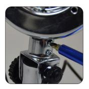
**4.** On the motor unit there is a clamp bracket with a tiny grub screw and a small black screw that will be used to adjust the vertical movement. Undo both these screws.
