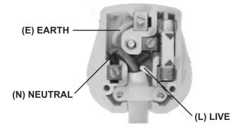
Your appliance operates on 220-240V~50Hz AC Mains and comes fitted with a 3-pin BSI Approved plug, so that it is ready for use for the UK or Eire market. If for any reason you need to fit a new plug, the flexible mains lead must be connected as shown below: -
