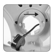
**GENTLY PLUG** the mains plug into the 220-240V ~ 50Hz AC mains outlet.
