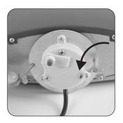
**1 REMOVE** the butterfly nuts from the lower part of the frame.
