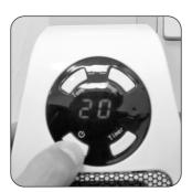
**8.** When finished, Press "  $\bigcirc$ " button, the heater will be off automatically in 1 minute, switch the power switch at the side of the heater to "Off" position and unplug heater from power outlet.
