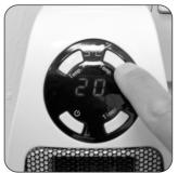
**5.** Press "Temp. -" button is for decreasing the temperature setting in High and Low mode.
