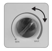
TURN the thermostat to its MAXIMUM POSITION. When the unit reaches the required temperature, TURN DOWN the thermostat, until the unit switches OFF. The temperature will now be kept CONSTANT. In its minimum position, the thermostat provides a 'Frost Watch' protection.
