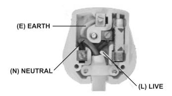
Your appliance operates on 220-240V~50Hz AC Mains and comes fitted with a 3-pin BSI Approved plug, so that it is ready for use for the UK or Eire market. If for any reason you need to fit a new plug, the flexible mains lead must be connected as shown below: -
