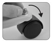
**2** FIT THE castor wheels by PLACING through the outer holes in the metal axle (bottom side) and SECURING with the enclosed bolts (top side). The flat side is the top of the axle.
