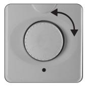
To determine the correct operating temperature your conditions, when for you first switch the unit on, TURN the thermostat to its MAXIMUM POSITION. When the unit reaches the required temperature, SLOWLY TURN **DOWN** the thermostat, until the unit SWITCHES OFF. The temperature will now be kept CONSTANT. When the temperature falls the unit will COME ON AGAIN.
