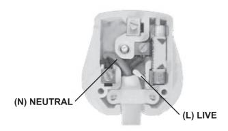
Your appliance operates on 220-240V~50Hz AC Mains and comes fitted with a 3-pin BSI Approved plug, so that it is ready for use for the UK or Eire market. If for any reason you need to fit a new plug, the flexible mains lead must be connected as shown below: -
