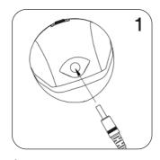
1. Insert the small plug into the charging socket at the bottom of (1), and the USB plug into any USB Charging adaptor or socket.
