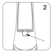
**2.** The indicator light (2) will illuminate when charging. When the appliance is fully charged (about 90 ins), the indicator light will turn off. Then you can use the appliance for approx. 90 mins.
