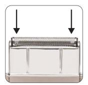
**4.** Replace the foil carefully by pushing the cleaned or new foil inside the head unit until they click into place.
