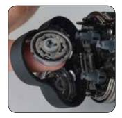
**3 REMOVE** all three Foil Heads and Cutting Blades by **GENTLY PUSHING** them through the underside of the Head Cover with your fingers. The Cutting Blades and Foil Heads will separate very easily. Care should be taken not to damage these components.
