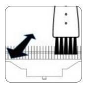
**4** USE the brush supplied to REMOVE any excess hairs or dirt from the blades. RINSE and DRY THOROUGHLY.
