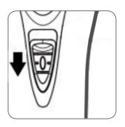
**4** PUSH the on/off switch to the 'OFF' position to DISENGAGE trimmer the blades.
