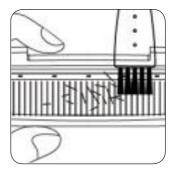
3 USE the brush supplied to REMOVE any excess hairs or dirt from the foil head. RINSE and DRY THOROUGHLY.
