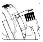
**PUSH** the trimmer switch to **EXPOSE** the trimmer and **GENTLY BRUSH** away any excess hair or dirt. **PULL** the trimmer switch **DOWNWARDS** to close after cleaning.
