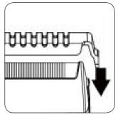
**9 PLACE** the plastic protective clip onto the head cover to protect the foils.
