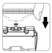
**6** CLIP the blades back into place on the spindle.
