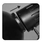
**4** ATTACH the lamp shade by **ALIGNING** the indents on the shade with the indents on the lamp holder. **TURN** the shade **CLOCKWISE** to **LOCK** it into position.
