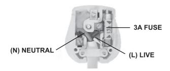
Your appliance operates on 220-240V~50Hz AC Mains and comes fitted with a 3-pin BSI Approved plug, so that it is ready for use by simply plugging into AC Mains. Should you need to change or refit a plug, proceed as follows: -
