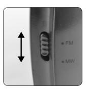
**2** TOGGLE between AM & FM on the band selector switch to CHOOSE between AM or FM wavebands
