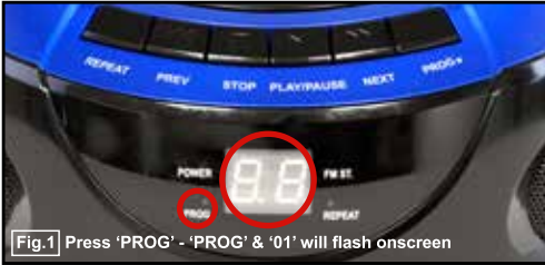
Fig.1 Press 'PROG' - 'PROG' & '01' will flash onscreen
